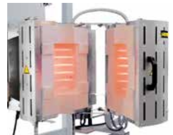
RS 100/250/11S in split-type design for integration into a test stand
