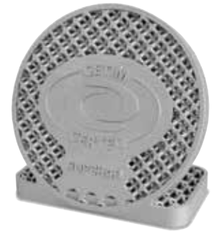
Printed aluminum part, heat treated in model N 250/85 HA (Manufacturer CETIM CERTEC on SUPCHAD platform)
