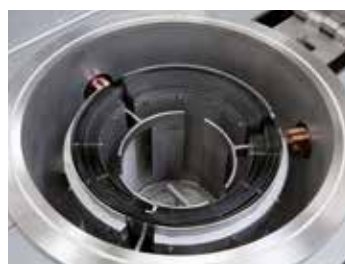
Cylindrical retort with tungsten heating
