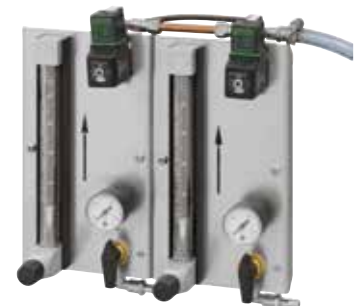
Two automatic gas supply systems, connected with each other
