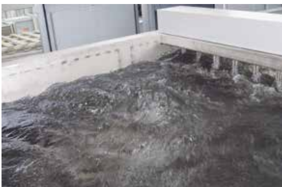
Powerful circulation of quenching medium
