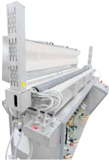
Wire annealing furnace based on a tube furnace with safety package for hydrogen as process gas
