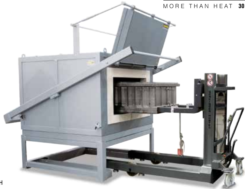
Chamber furnace N 321 with charging stacker
