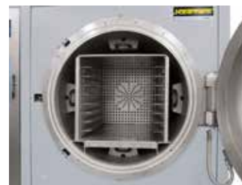
Retort with internal heating
