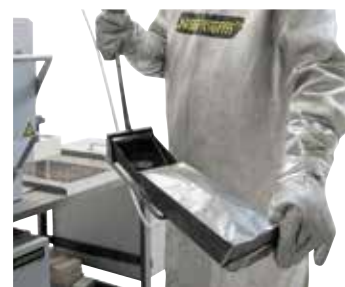
Protective gas annealing bag in operation
