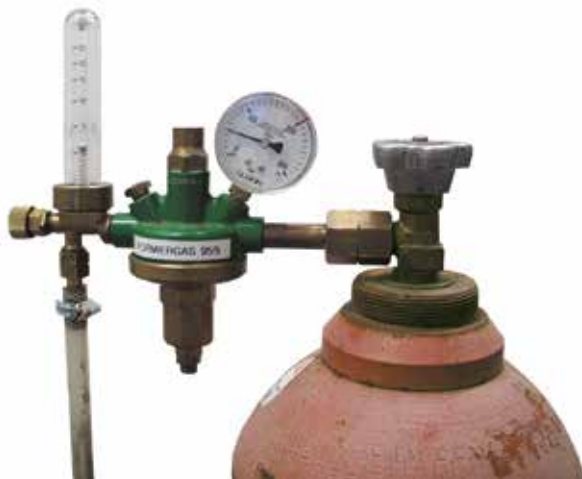
Pressure reducing valve with assembled flow meter
