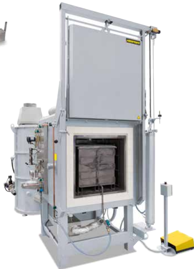
Air circulation chamber furnace N 250/65 HA IDB with protective gas box for inert debinding under protective gases incl thermal post combustion (TNV). Please also see catalog Advanced Materials.
