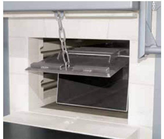
Protective gas box with flap which opens together with the furnace door
