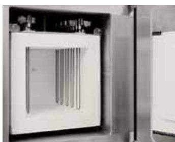
Molybdenumdisilicide heater and fiber insulation
