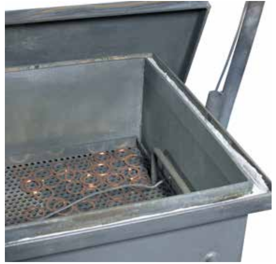
Heat treatment under protective gas atmosphere in a protective gas box incl. charge thermocouple
