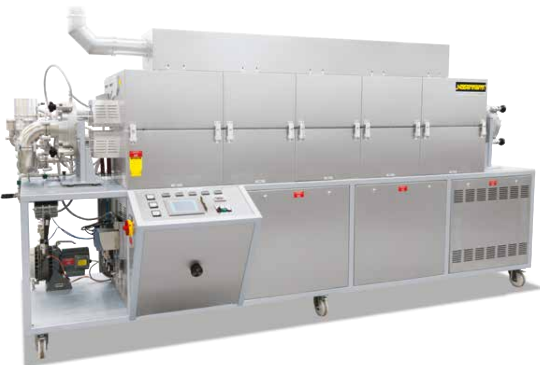
RS 250/2500/11S, five-zone controlled, for wire annealing in high-vacuum or under protective gases, incl. forced cooling and exhaust hood
