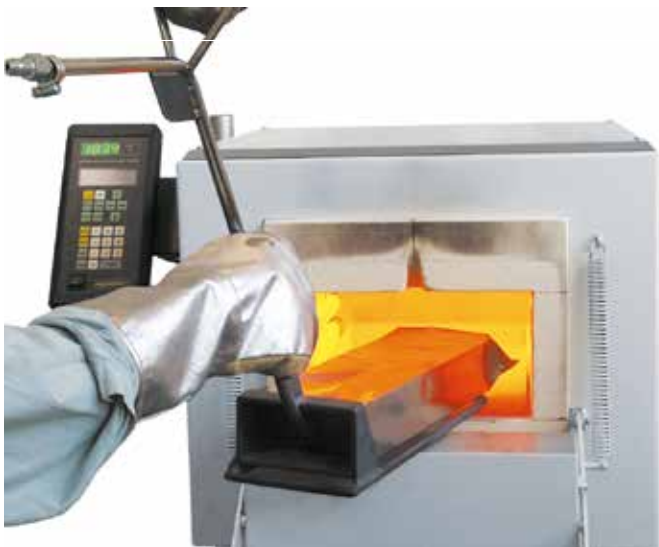
Hardening in annealing tray with alloy bag
