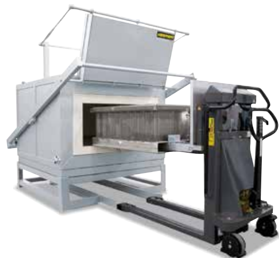
Charging stacker WS 641 with chamber furnace N 641 and guiding track at the base frame
