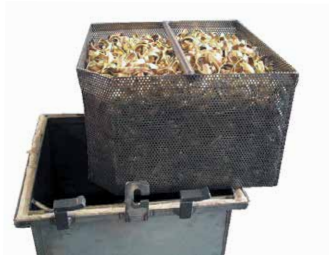
Bulk material bright annealing in an annealing box with evacuation facility
